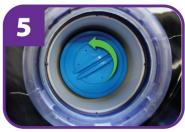
Remove filter by turning counter-clockwise. Remove plastic filter transport bag.
