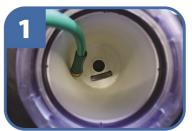
Place fill hose into open filter canister When filled all massage jets should be and fill spa until water is 5" (12.5cm) from the top "lip" of the hot tub.
