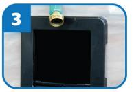
Remove fill hose from filter canister.
