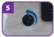
Loosen (do not remove) the air bleeder valve by turning counterclockwise.
